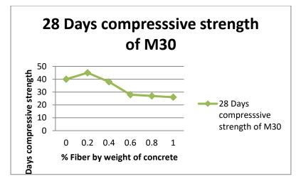
These results show that compressive strength of concrete increases just at 0.2% fibres. It is because at this fibre content it fills the voids. It is also seen that compressive strength of concrete reduces drastically when fibres content is increased beyond 0.2%. The amount of gain of compressive strength is shown in table below: -
