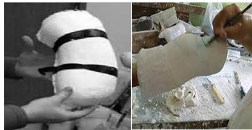
Figure 2.b. positive mould by filling POP and socket rectification by adding and removing POP.
