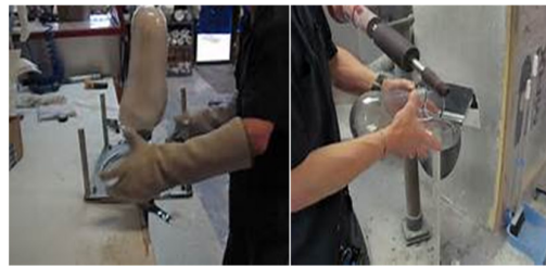
Figure 2.c. socket preparation by lamination and final trimming
