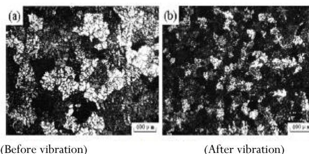
Figure.2. SEM Analysis of AZ80 alloy
