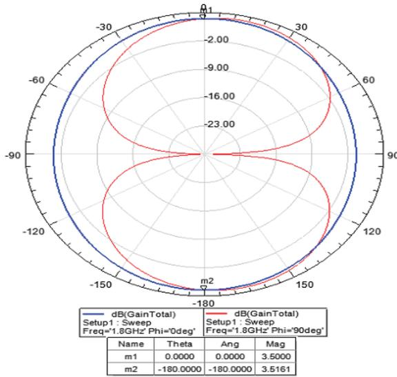
Figure 7: Radiation pattern at 1.8 GHz.
