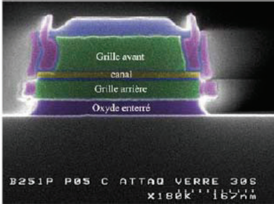
Figure 2. DG MOSFET structure under Scanning Electron Microscopy [7].
