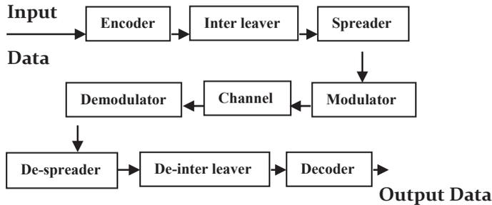
Fig.2 Basic Block Diagram for the proposed scheme
