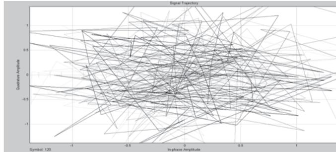
Fig.15 Signal trajectory of I- and Q- components with AWGN + Rayleigh/Rician fading for RS (7, 3) code (M=2)
