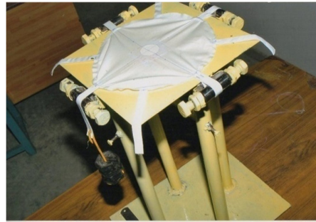
Fig 1. (a). Newly developed bi-axial stress & strain tester (BASS)
