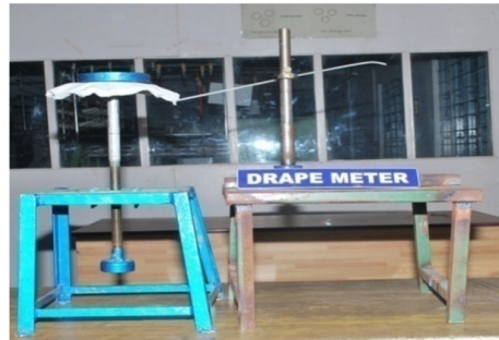
Fig 1. (b). newly developed drape & stiffness tester (DST)
