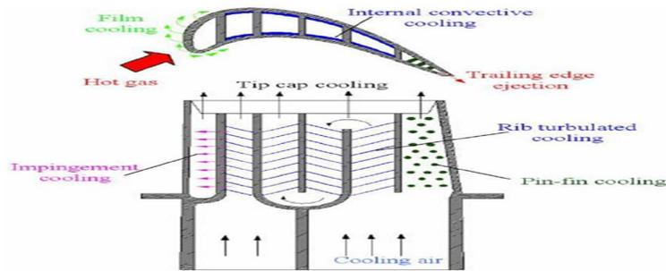
Figure 1: Typical cooling techniques of turbine blade
