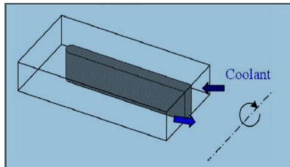
Figure 2: Two pass serpentine passages inside a turbine blade [2]
