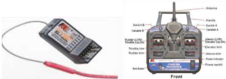
Fig 7: Receiver and Remote Control
