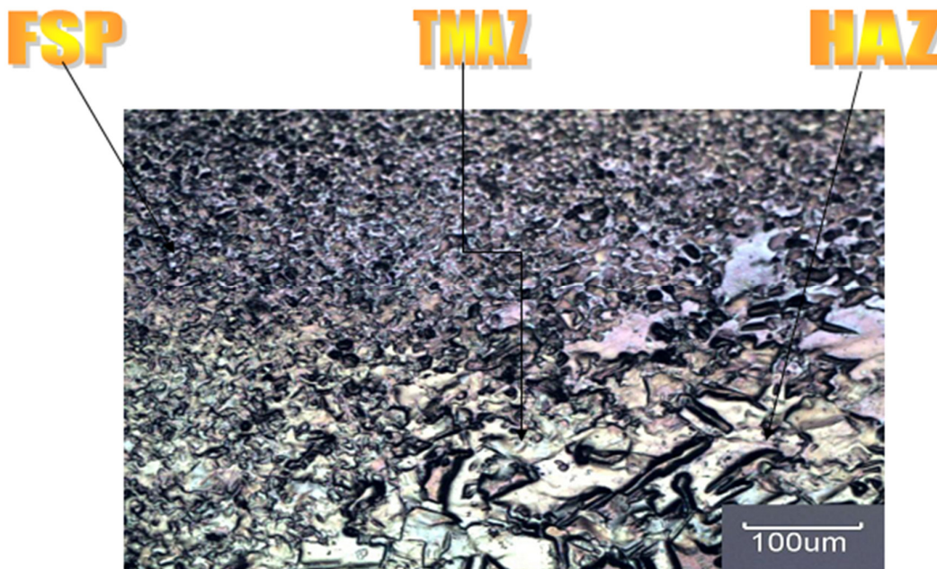
Fig 4.1 Optical Photomicrograph of Transient Zone between Cu and AlN
