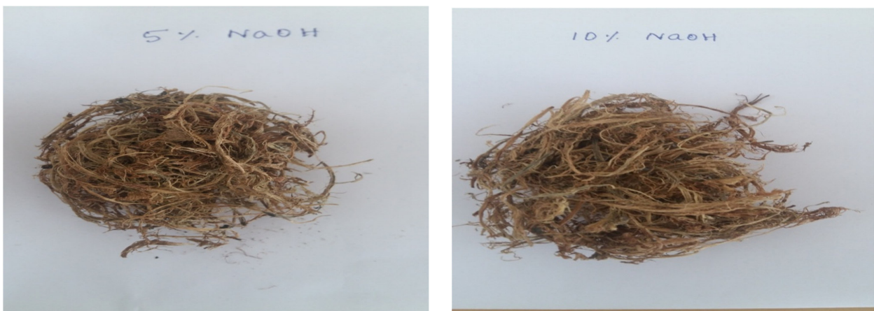
Figure 2. 5% and 10% NaOH alkali treated Terminalia Catappa fruit fibers
