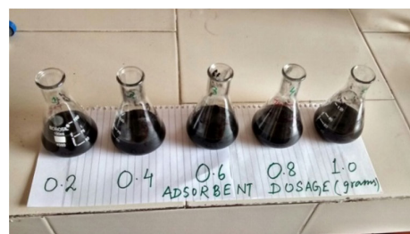
Figure 2. Foundry effluent being treated with different adsorbent dosages
