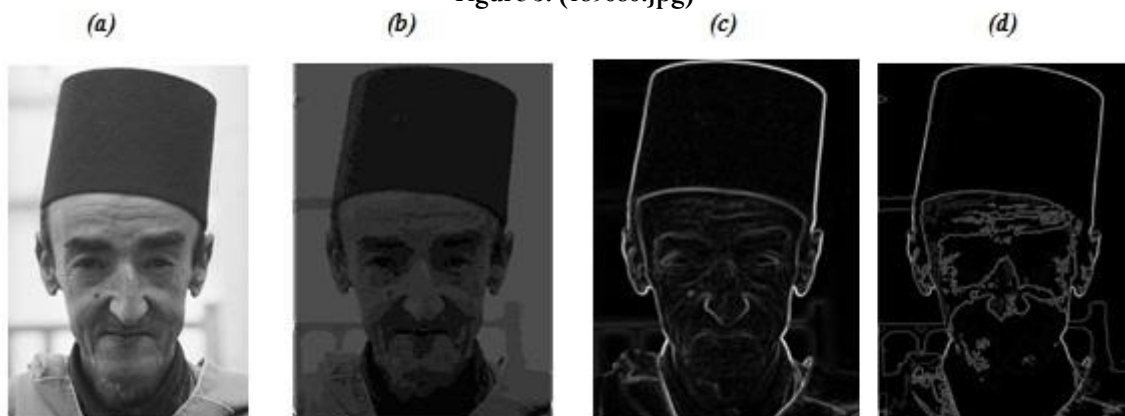
Edge detection: (a) input image, (b) K-means clustered image, (c) Gabor Wavelet image, (d) Both K-means clustering and Gabor Wavelet
