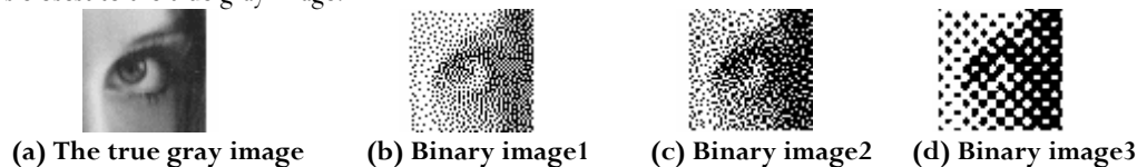
Fig. 6: Basic principle of halftone technique
