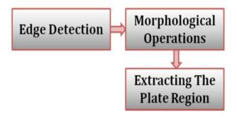
In this stage, the location of the license plate is identified and the output of this stage will be a sub-image that contains only the license plate. This is done in two main steps.
