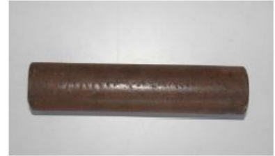
Figure 7(b) Final State of metallic structure with no protection.
