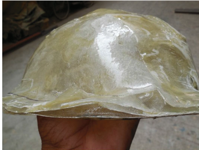
Figure 5. Fiber Glass Helmet after Removing From the Mould
