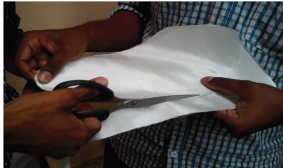
Figure2. Cutting the Glass Fiber Cloth To Get the Desired Shape
