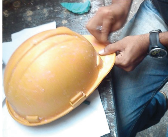
Figure 3. Applying Wax on the Mould
