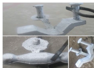
Fig.6.2 Castings produced when fired with coke and diesel
