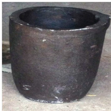
Fig.3.1. Clay graphite crucible
