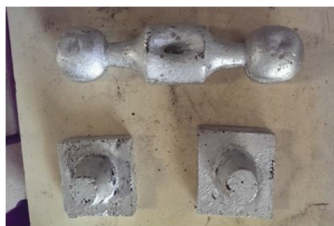
Fig.6.1 Castings produced when fired with coke
