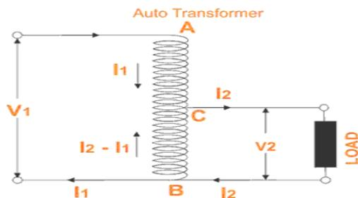
$\frac{V_1}{N_1} \times N_2$  and from the figure above, this voltage is  $V_2$ .
