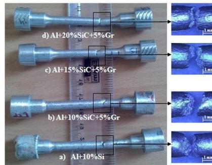
Fig. 2 Tensile tested specimen with different type of fracture
