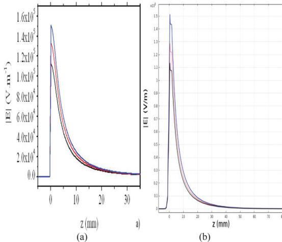
Figure 6. Norm of electric field  $|E|$  on the axis ( $r = 0$  mm) for powers of 500 W (black curve), 700 W (red curve) and 900 W (blue curve). The frequency delivered is 2.45 GHz. (a) obtain with our calculations, (b) Obtain by [3]
