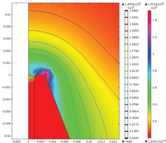
Figure 5. Distribution of the electric field around the nozzle
