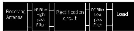
**Figure 1:** Block diagram of a conventional rectenna.
