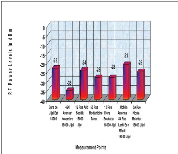
Figure 4: Measurements of power density at different points in Jijel.
