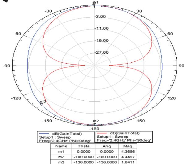
Figure 10: Radiation pattern at 2.4 GHz.
