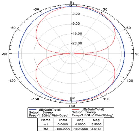
Figure 7: Radiation pattern at 1.8 GHz.
