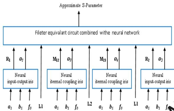
Figure 3. Structure for the three cavity waveguide filter, with four neural-network sub-models.
