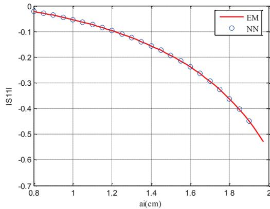
Figure 2. Variation of iris response against ai at fixed frequency and iris length
