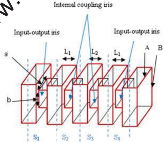
Figure 1. Geometry and segmentation of rectangular waveguide three cavities.
