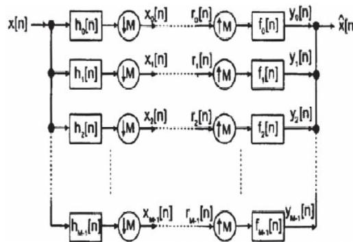
Fig. 1. M-Channel maximally decimated filter bank.
